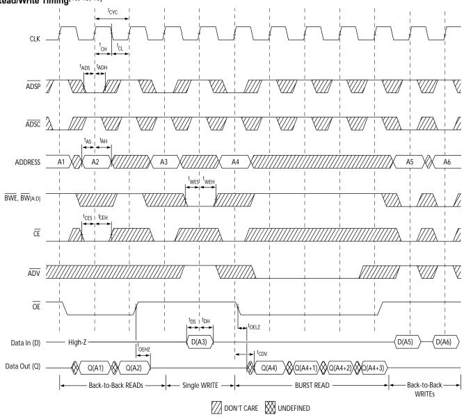
Notes: 18. <u>The</u> data bus (Q) remains in High-Z following a Write cycle unless an <u>ADSP</u>, <u>ADSC</u>, or <u>ADV</u> cycle is performed. 19. <u>GW</u> is HIGH.
